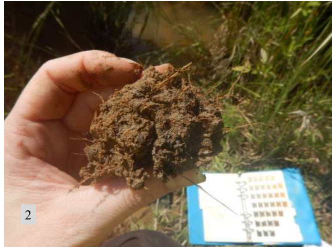
▲ DP 1—Hydric soil with a depleted matrix was observed at DP 1 within Wetland 1.
