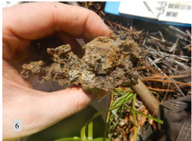
▲ DP 4—Hydric soil with a depleted matrix was observed at DP 4 within Wetland 2.
