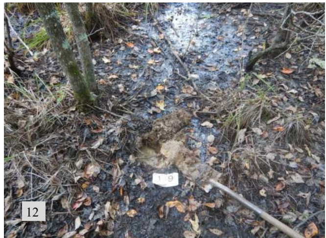
▲ DP 19—Soil within Wetland 4 met hydric soil criteria as the wetland exhibited a hydrogen sulfide odor.
